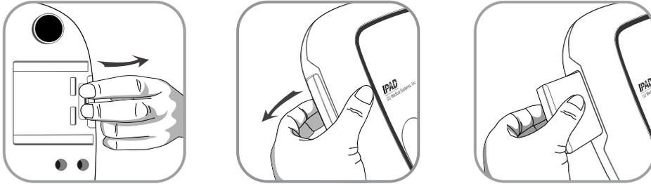
2. Insert a new battery pack in the direction of the arrow with the label facing upward as shown in the figure below.
