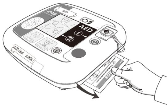
3. Insert the pads connector of the new pads into the Defibrillator Pads Connector , and then put the pads package in the Pads Storage Compartment as illustrated below.
