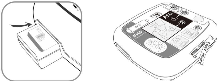
As the battery pack is inserted, the device starts a self-test. If the device status is normal, **○** is shown on the Status LCD. If **✘**, **□** or **□** is displayed on the Status LCD after the self-test, please refer to [Chapter 8: Troubleshooting] of these Instructions for Use.
