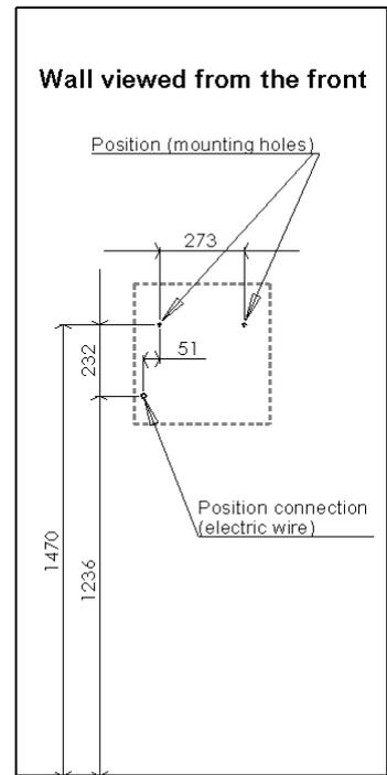
2. The Cabinet should be mounted onto the wall or stand with screws attached through the 2 holes in the back panel.
