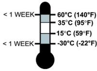
Recommended storage temperature: 15° to 35°C (59° to 95°F). Storage at extreme temperatures of -30° and 60°C (-22° and 140°F) is limited to seven days. If storage at these temperatures exceeds one week, the electrode shelf-life will be reduced.
