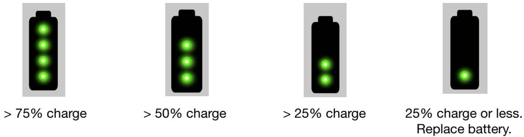
Figure 2-3 Battery Charge Indicators
