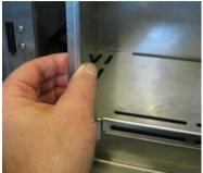
There will now be free access to the section of the unit where phase, neutral and ground wires are to be connected.
