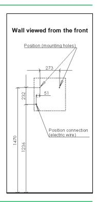
The Cabinet should be mounted onto the wall or stand with screws attached through the 2 holes in the back panel.
